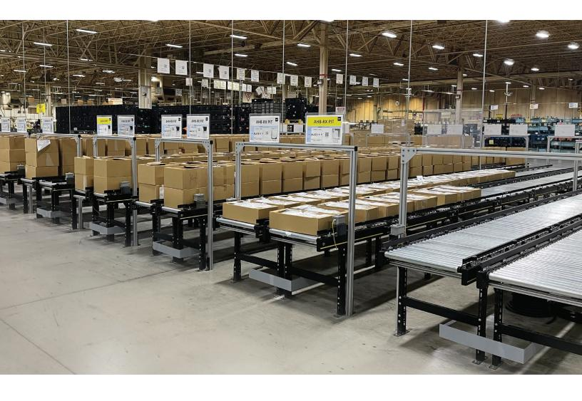
Zero pressure accumulation (ZPA) conveyors do not allow products to touch each other, while conveying, thus reducing back pressure and damage to product during accumulation. ZPA conveyors can be used to stage products in specific zones to complete a process or accumulate in zones while product is moved down the line.
